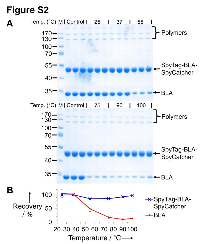
**SpyTag-BLA-SpyCatcher stability was retained after mixing with BLA.** a) SpyTag-BLA-SpyCatcher was mixed with BLA, heated at the indicated temperature for 10 min, centrifuged and the supernatant analyzed by SDS-PAGE with Coomassie staining. M: molecular weight markers. Triplicate samples are shown. The control was without any incubation. b) Quantification of soluble fractions from a) (mean of triplicate ± 1 s.d.). Some error bars are too small to be visible.
