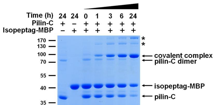
**Figure S6.** Time-course of spontaneous amide bond formation by SDS-PAGE. Isopeptag-MBP and pilin-C were mixed at 10  $\mu$ M and incubated at 25  $^{\circ}$ C, pH 7.0. The reaction was stopped at varying times and analyzed by SDS-PAGE with Coomassie staining. \*This side-product likely relates to the pilin-C dimer reacting with 1 or 2 isopeptag-MBP.
